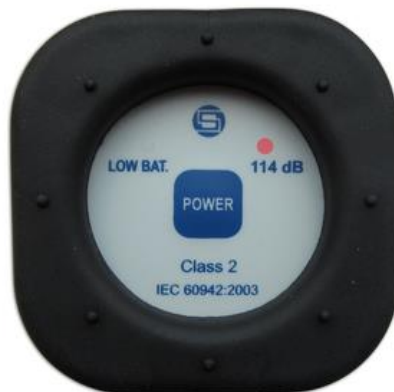
Picture 4. The top view of the SV 34B calibrator with one diode on
