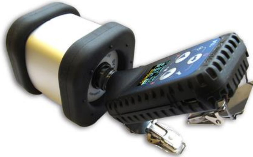
Picture 2. Calibration of the personal exposure meter with a ½” measurement microphone
