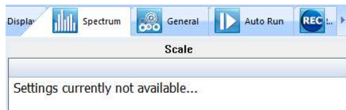
Figure 6-9 Example of a category of settings unavailable due to some other options in the same setup file being disabled
