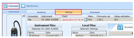
5) Download current Settings from Instrument files to Local Files using right arrow and edit SV103 settings using panels on the right hand side
