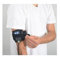
4) Place the SV 107B on the palm of the hand as shown below. Secure the cable on a wrist with a wrist band.
